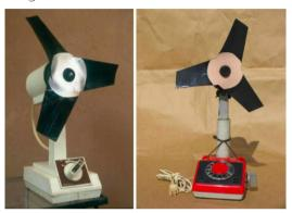
Image 3 - Fan with Russian washing machine engine Aurika 70.
