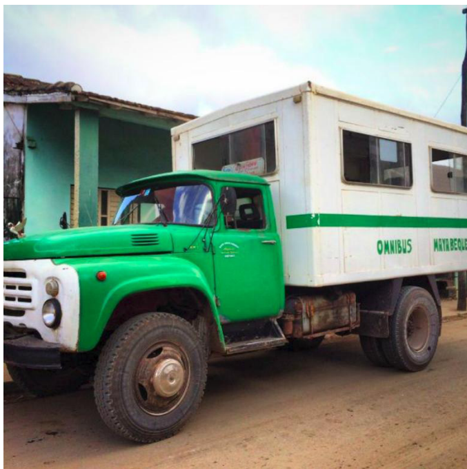
Image 6 - Bus made with parts of a truck.
