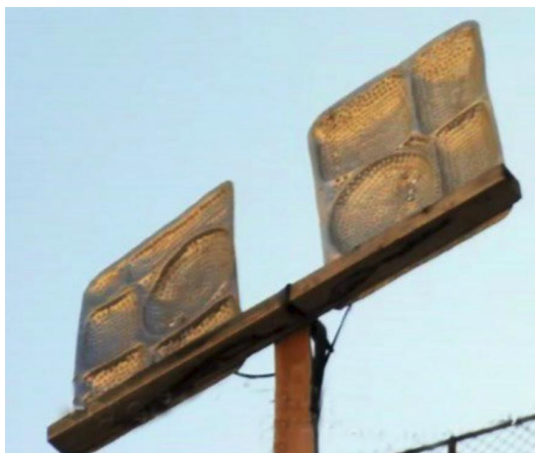
Image 8 - TV antenna made with aluminum trays.
