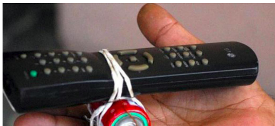
Image 9 - Remote control with battery adaptation.
